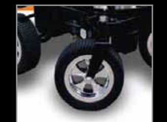
Flat-Free Swivel Wheel: 360° swivel flat-free mag style tire and wheel assemblies for the best mobility available.
