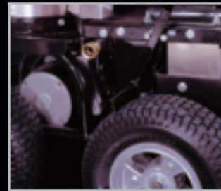
Brake Assembly: Two wheel locking brake assembly. Correctly conforms to ETL Listing requirements.
